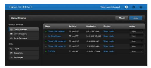
3. The view pane lists the available streams. For this example, we are going to add a stream that uses TS over SRT. Click the +Add button. *If you have an existing SRT stream, you can modify it instead.*
