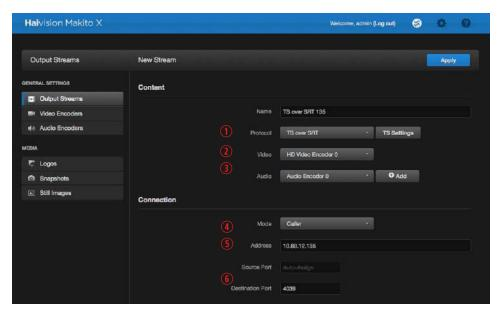
5. Under the Connection section, specify the 4 mode as "Caller," enter the 5 address for the Media Gateway (in the Cloud) and a 6 Destination port.
