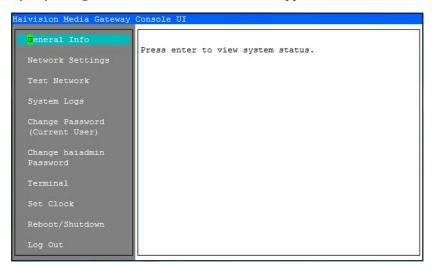
The navigation sidebar (left pane) provides the menu/action items. The right pane displays a detailed view of the selected item. To control the Console UI:
