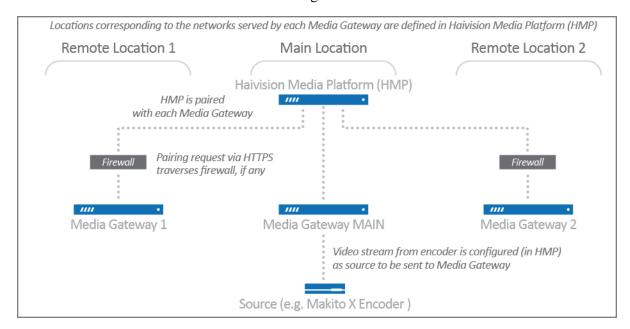
In Media Platform, you also need to establish a connection between the video source (for example, a Makito X Encoder) and one of the paired Media Gateways.
