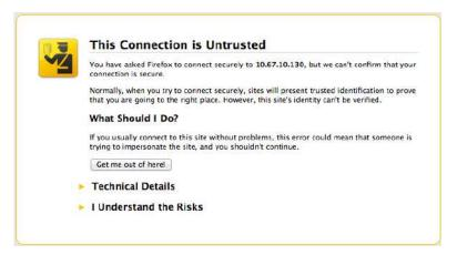
Supplying the Media Gateway with an SSL security certificate eliminates the security warning, provides a means for users to verify a website, and ensures that the connection is secure. See "Certificates" on page 86 for more details.
