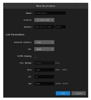
Checking the Traffic Shaping checkbox allows you to manually adjust the maximum bitrate. Traffic Shaping controls the outgoing stream so that the interpacket time is constrained, in order to reduce the probability that TCP packets are dropped in a session.
